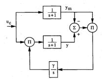
Fig. 1 Block diagram of the adaptive system.
